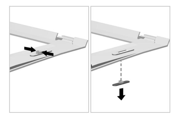
Figure 5-35. Removing a Brightness/Contrast Control Actuator
